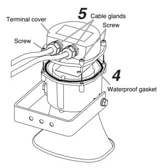
Step 7. Securely tighten the cable glands.
