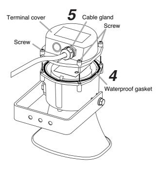
Step 5. Securely tighten the cable gland.
