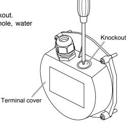
Step 2. Attach the cable gland to be added.
