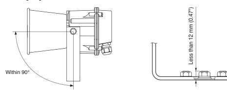
• Do not install the speaker face-up from a horizontal plane. If water accumulates in the horn, this may cause the speaker malfunction.
